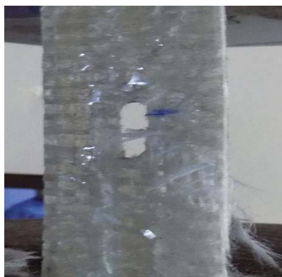
Fig. 7. Composite plate with single hole – Failed specimen
